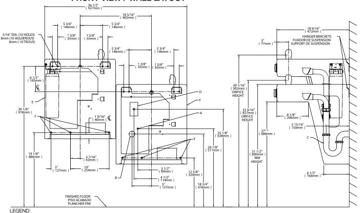
A = RECOMMENDED WATER SUPPLY LOCATION. SHUT OFF VALVE (NOT FURNISHED) TO ACCEPT 3/8" O.D. UNPLATED COPPER TUBE.
